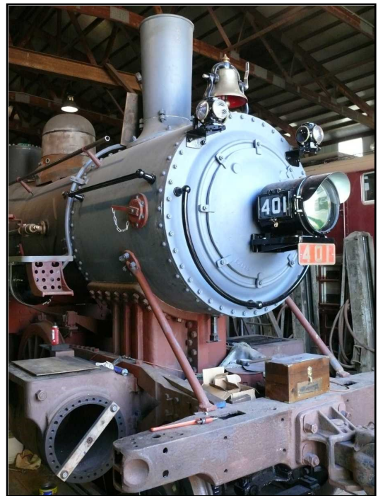
Southern 401 is coming to life with the application of headlight, bell and classification lights.
