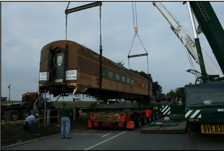
Diner ICRR 4112 is being lifted off its trucks and onto a trailer for movement between LASM and CN Yard . Photo courtesy of John Fortner-SELA-NRHS
