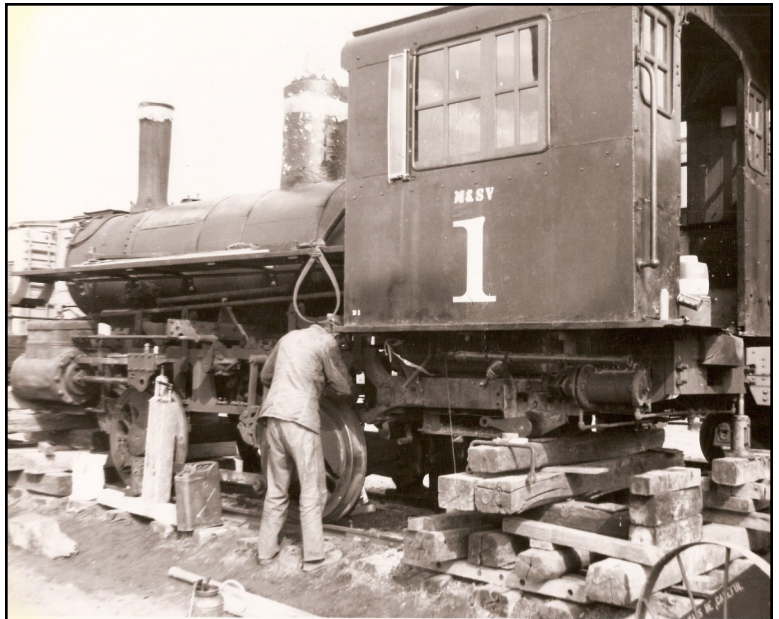
“Little Dumpy” soon found a new home in the Camp Creek Yards and in the “open air” shop” receives repairs to keep the locomotive in operating condition
