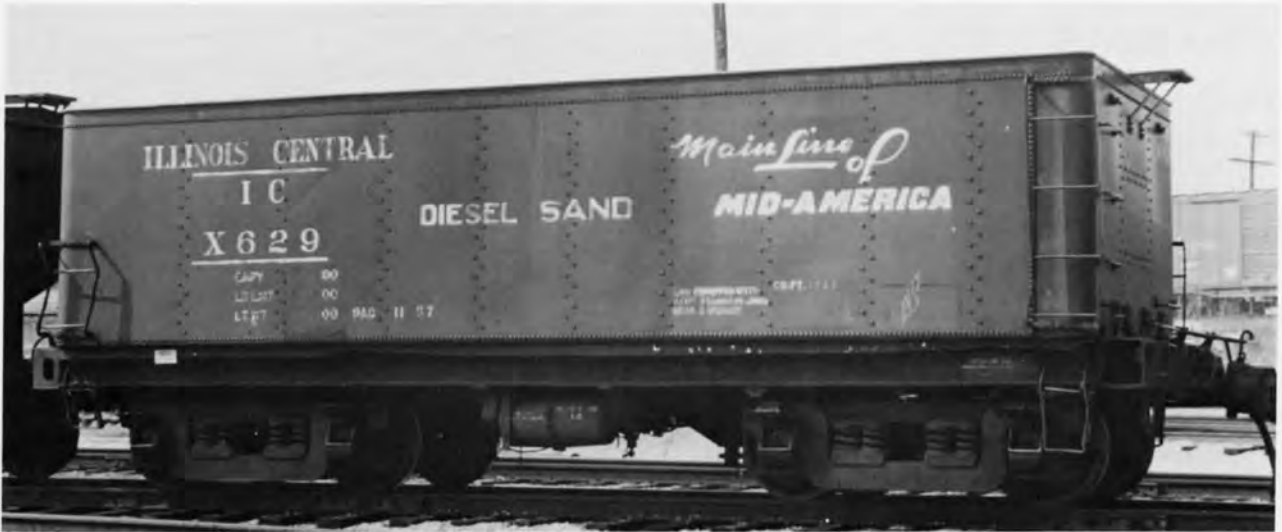
IC X629 SAND CAR. PHOTO BY BRUCE MEYER. Former IC water car. These cars were built by the IC and rebuilt by the Paducah, KY locomotive shop for diesel sand service, diesel fuel service or a combination of both.
