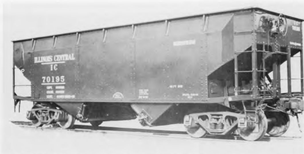
IC 70195 HOPPER. PHOTO ACF - ICHS COLLECTION. The 70000-70499 series cars built by ACF in 1948 in St. Louis, MO. The 50 ton copy cars were assigned mainly to coal service in Southern Illinois and Kentucky.
