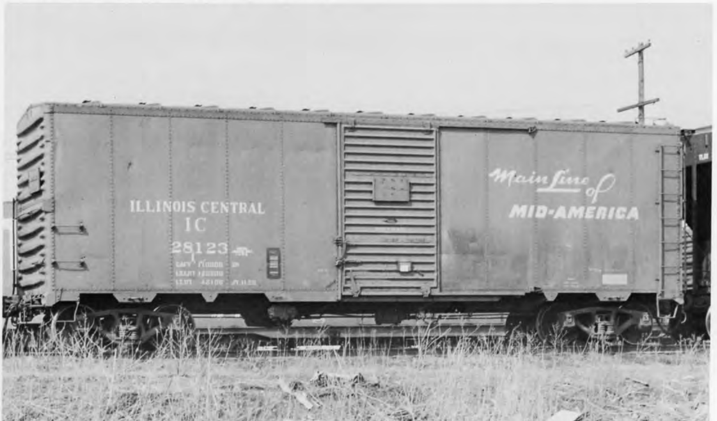
IC 28123 BOXCAR 40FT. PHOTO BY BRUCE MEYER. The 28000-28999 series cars were built by G.A.T. in 1940. Several cars in the series were rebuilt by the IC Johnson yard car shop at Memphis, TN in 1966. Several cars were assigned for cotton loading only.
