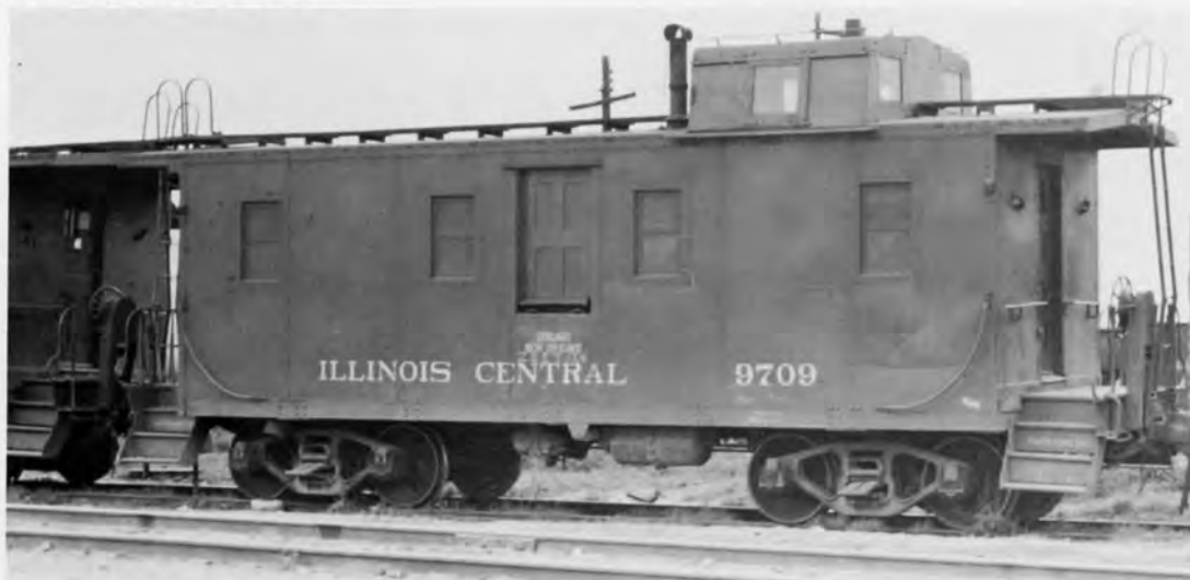
IC 9709 CABOOSE. PHOTO BY JAY WILLIAMS. The 9701-9799 series cabooses were built by the IC Centralia, IL car shop in 1940.
