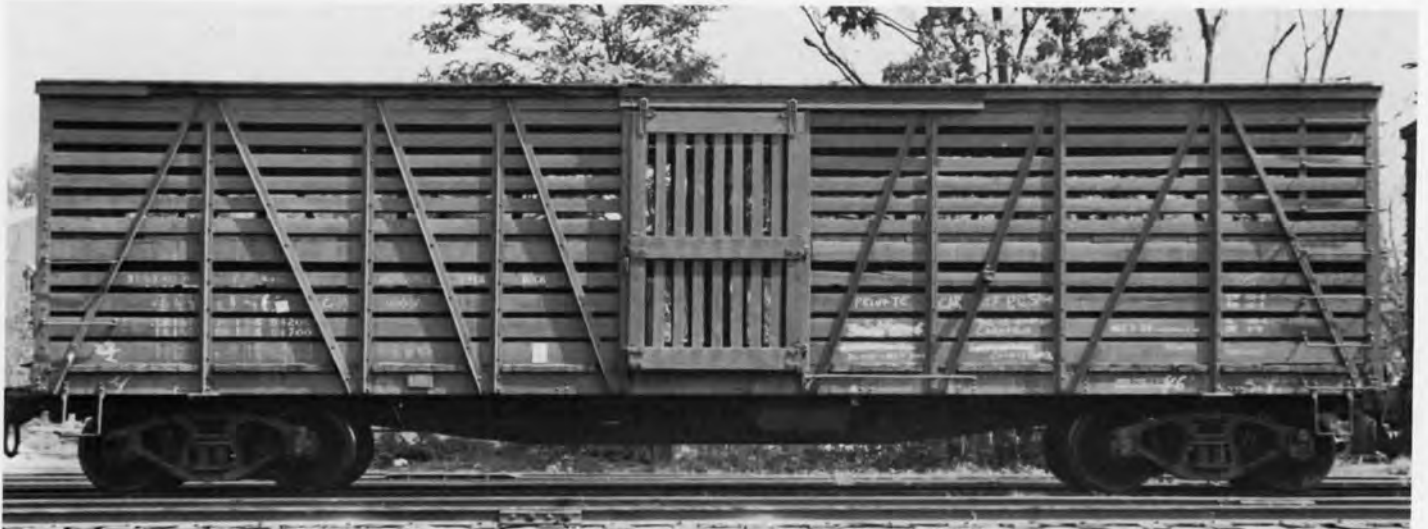
IC 46086 STOCK CAR. PHOTO BY BRUCE MEYER - ICHS COLLECTION. The 46000-46199 were built by General American Car Co. in 1925 & 1926 as 31001-31200 cars. Rebuilt by IC McComb car shops in 1952 and renumbered to 46000-46199 series.
