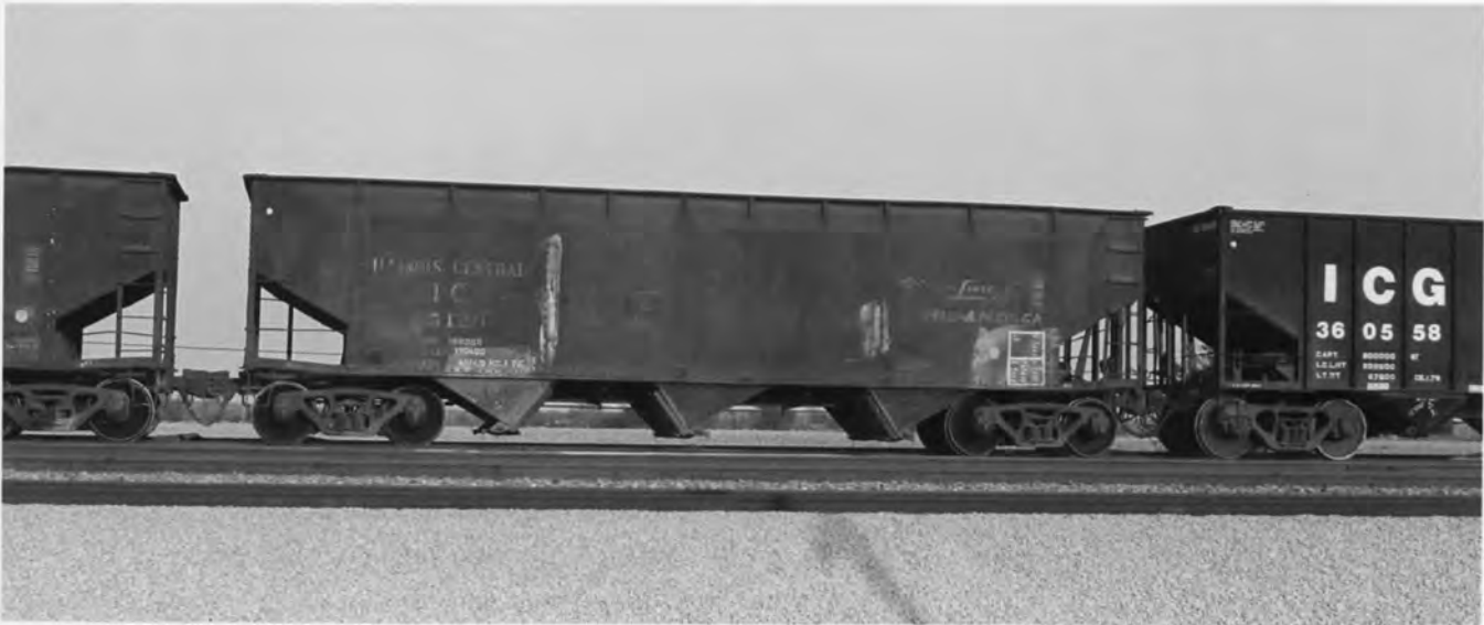
IC 65120. HOPPER. 65000-67999. ICRR 1964. 70 ton capacity.
