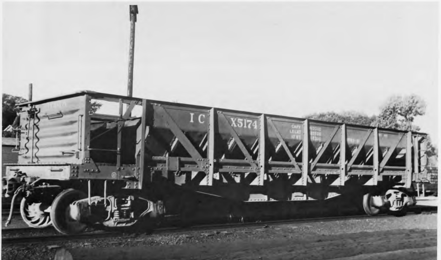
IC X5174 BALLAST CAR. PHOTO G.V. CARSON - ICHS COLLECTION. The X5100-X5299 series 50 ton ballast cars were built by ACF in 1923 and were originally numbered 113401-113900.
