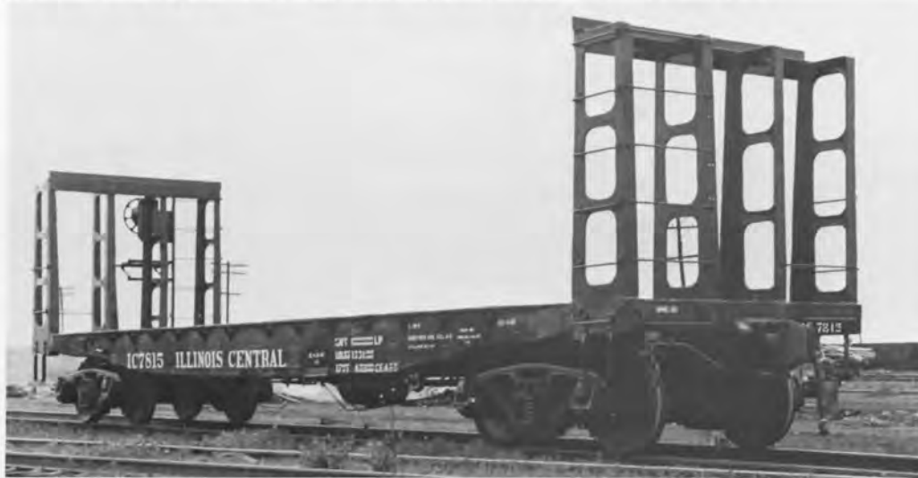
IC 7815 FLAT. PHOTO ICRR - ICHS COLLECTION. The 7800-7837 series cars were built by the IC Centralia, IL car shop in 1963. The 50 ton, 38 ft flat cars were assigned to pulpwood loading. The underframe and end bulkhead are cast steel by General Steel Casting Co.
