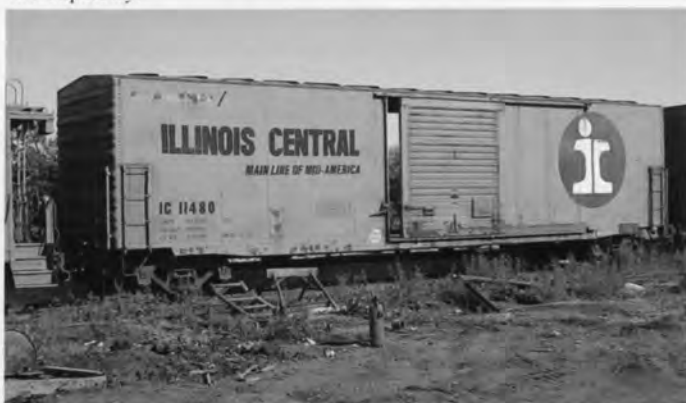
IC 11480. 50FT BOXCAR. 11300-11499. ACF 1967. 70 ton capacity.
