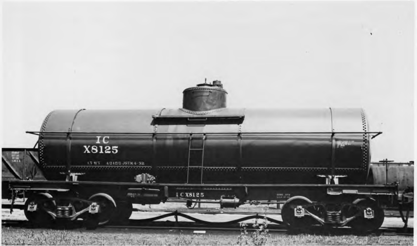
IC X8125 TANK CAR. PHOTO BY G.V. CARSON - ICHS COLLECTION. The X8125-X8129 series tank cars were built by ACF in 1905 for the IC and originally numbered 1-5.
