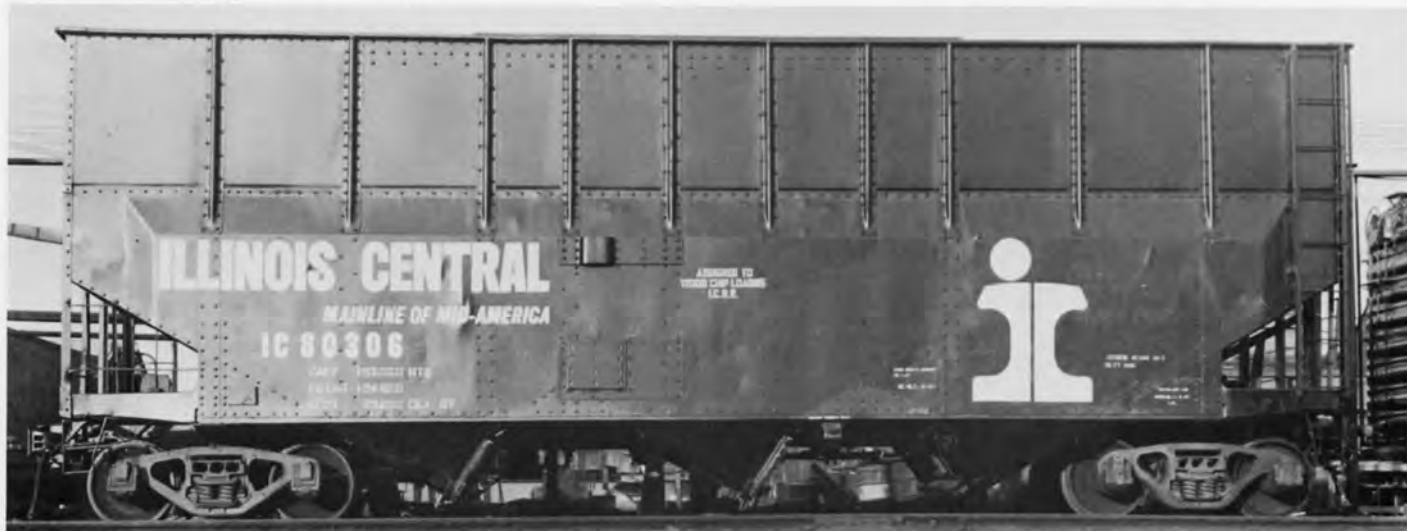
IC 80306 HOPPER. PHOTO BY ICRR - ICHS COLLECTION. The 80300-80499 series cars were built by the IC Centralia car shop in 1967. The 70 ton copy cars were assigned to wood chip loading only.
