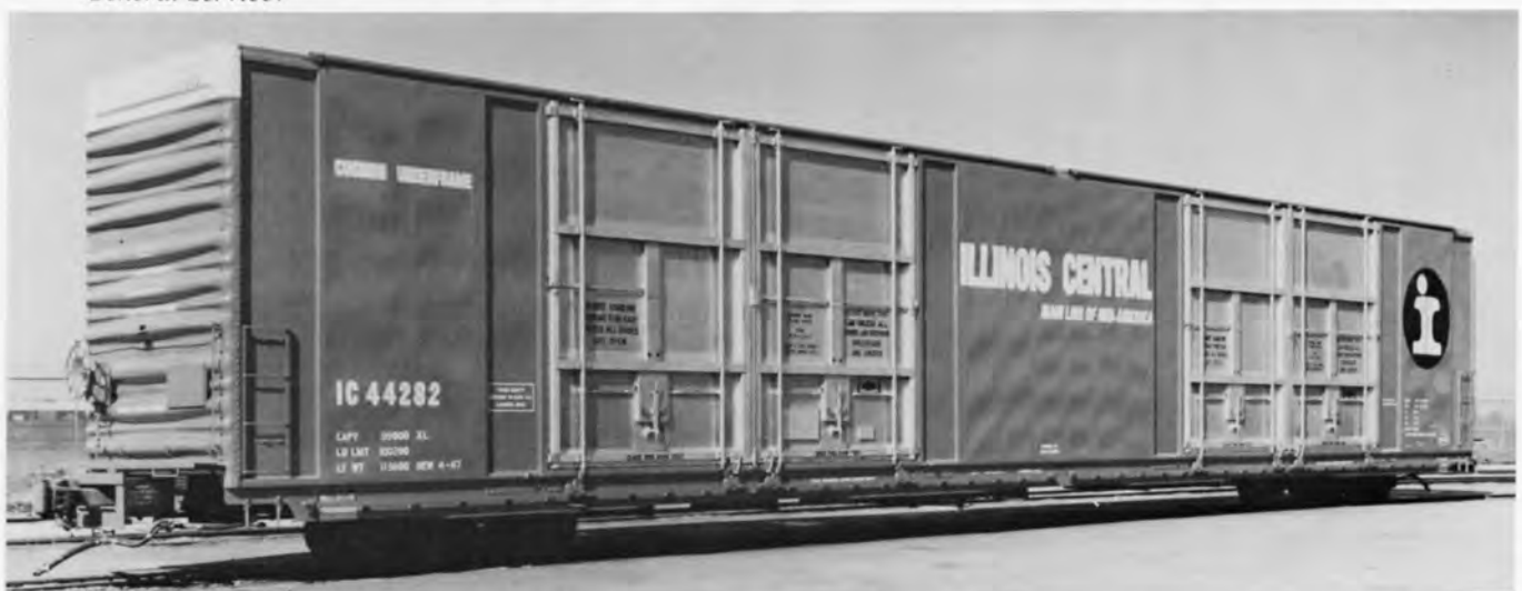
IC 44282 HI-CUBE BOXCAR 86FT. PHOTO ICRR - ICHS COLLECTION. The 44282-44285 series cars were built by Thrall in 1967. Equipped with 2 movable bulkheads and 5 belt rail DF-2 load devices. These cars were assigned to auto parts service.
