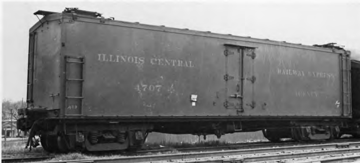
IC 4707 REEFER. PHOTO BY G.V. CARSON - ICHS COLLECTION. Steel frame express reefer with plywood sides and ends.
