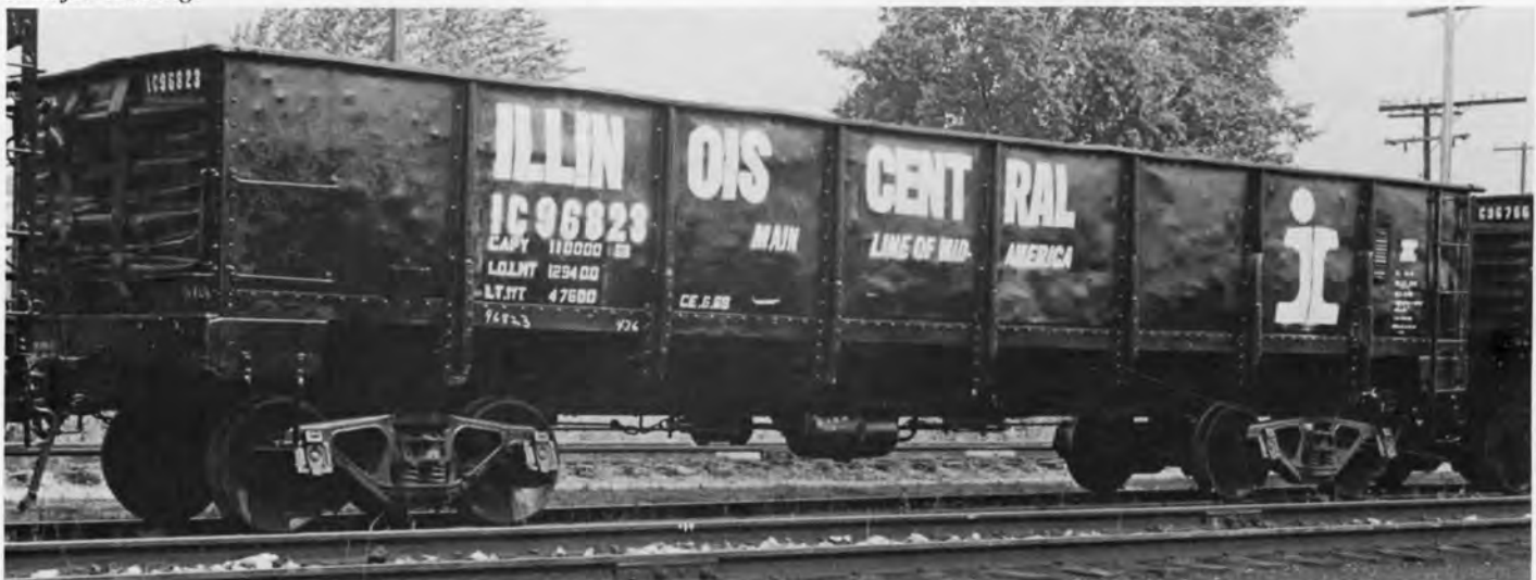
IC 96823 GONDOLA. PHOTO BY ICRR - ICHS COLLECTION. The 96000-96929 series 41 ft, 50 ton solid bottom general service gondolas were rebuilt by the IC Centralia, IL and McComb, MS car shops in 1967 & 1968 from the former 94000-95499 series drop bottom equipped cars.
