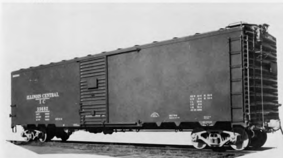
IC 33682 BOXCAR 50 FT SD. PHOTO BY ACF - ICHS COLLECTION. The 33500-33999 series cars were built by ACF in 1941 at their St. Louis, MO plant. Cars assigned to auto parts service.
