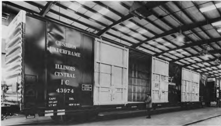
IC 43974 HI-CUBE BOXCAR 86FT. PHOTO BY ICRR - ICHS COLLECTION. The 43970-43999 series cars were built by Thrall in 1964. Cars are equipped with movable bulkheads and DF-2 belt rails. The cars were assigned to the GTW RR for loading at Flint, Michigan for auto parts service.
