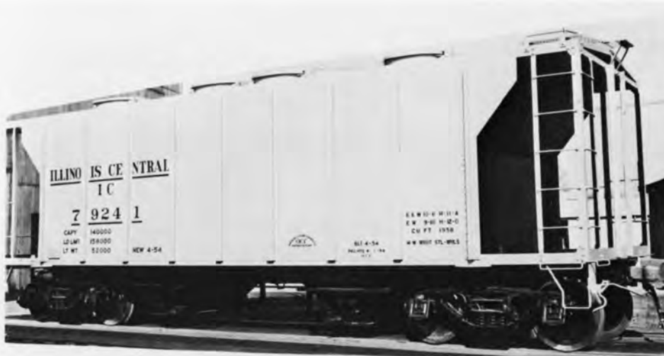
IC 79241 COVERED HOPPER PHOTO BY ACF - ICHS COLLECTION. The 79200-79299 series cars were built by ACF in 1954 with 70 ton capy.
