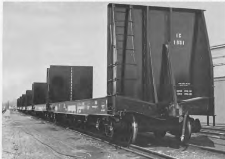
IC 1951 FLAT. PHOTO BY IC CENTRALIA CAR SHOP EMPLOYEES - ICHS COLLECTION. The 1000-1999 series cars were built in 1967 by the IC. The cars are 50 ft long with 70 ton capy. Cars are assigned to pulpwood loading.
