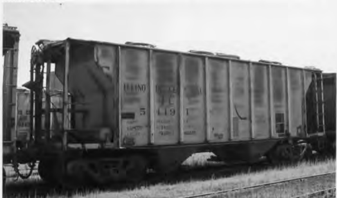
IC 54191. COVERED HOPPER. 54150-54299. ACF 1960. 70 ton capacity.
