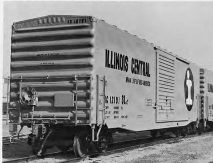
IC 12191 BOXCAR 50FT. PHOTO ICRR - ICHS COLLECTION. This car is part of the 12100 to 12622 series built by Pullman Standard in 1967. The cars are equipped with nailable steel floors, 4 SL-2 belt rails and loading strap anchors at the doorways.
