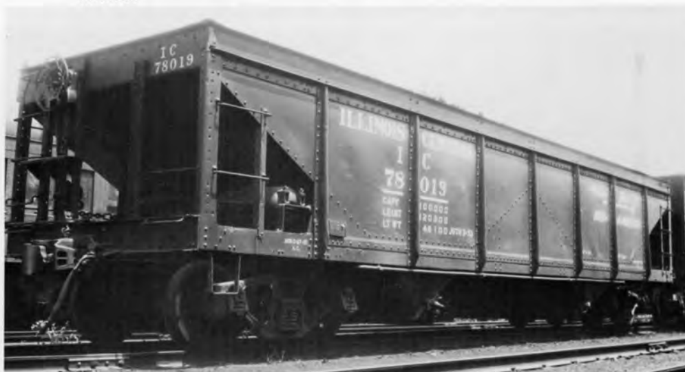
IC 78019 HOPPER. PHOTO G.V. CARSON - ICHS COLLECTION. The 77000-78965 series cars were rebuilt by the IC in 1946 & 1947 from former 90000-93970 hoppers built in 1921.
