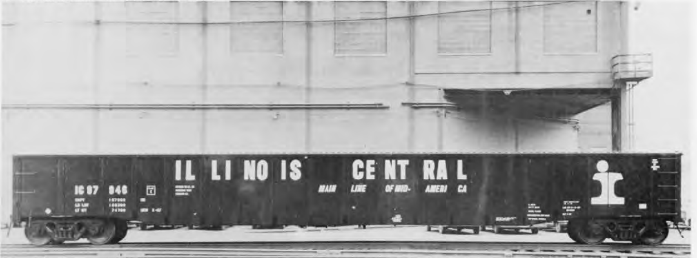
IC 97946 MILL GONDOLA. PHOTO BY ICRR - ICHS COLLECTION. The 97900-97999 series mill gondolas were built by Bethlehem in 1967. The cars are 100 ton capy equipped with dreadnaught drop end doors, continuous lading band anchor on top rail of sides and 12 4x4 timber post on the inside side walls (6 per side).
