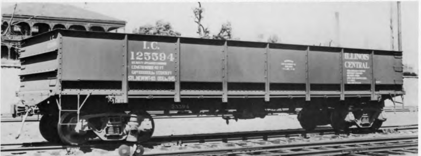
IC 125594 GONDOLA. PHOTO ACF - ICHS COLLECTION. Built in 1915 by ACF. Equipped with side dump.
