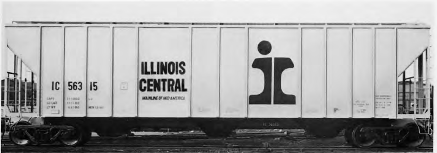
IC 56315 COVERED HOPPER. PHOTO BY ICRR - ICHS COLLECTION. The 56300-56799 series of covered hoppers were built by G.A.T.X. in 1966 & 1967 at E. Chicago, IN. The cars are 100 ton capy with 4700 cu ft capy. The cars are equipped with a 3 piece 44 ft hatch. These cars are assigned mainly to grain service.
