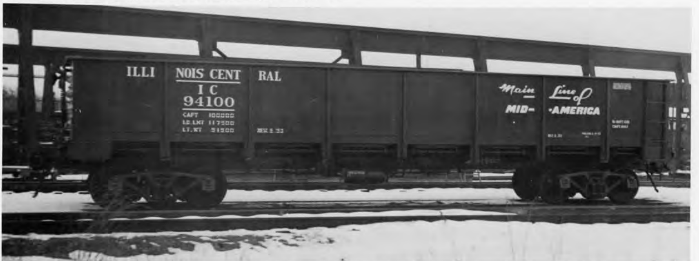
IC 94100 GONDOLA. PHOTO ICRR - DAVID J. DAISY COLLECTION. The 94000-95499 series cars were built by the IC Centralia, IL car shop in 1953. The cars are 50 ton capy and equipped with drop bottoms. Cars were converted to solid bottoms in the 1960s.
