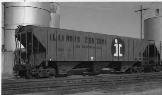
IC 57176. COVERED HOPPER. 56500-57199. Pullman Standard 1969.
