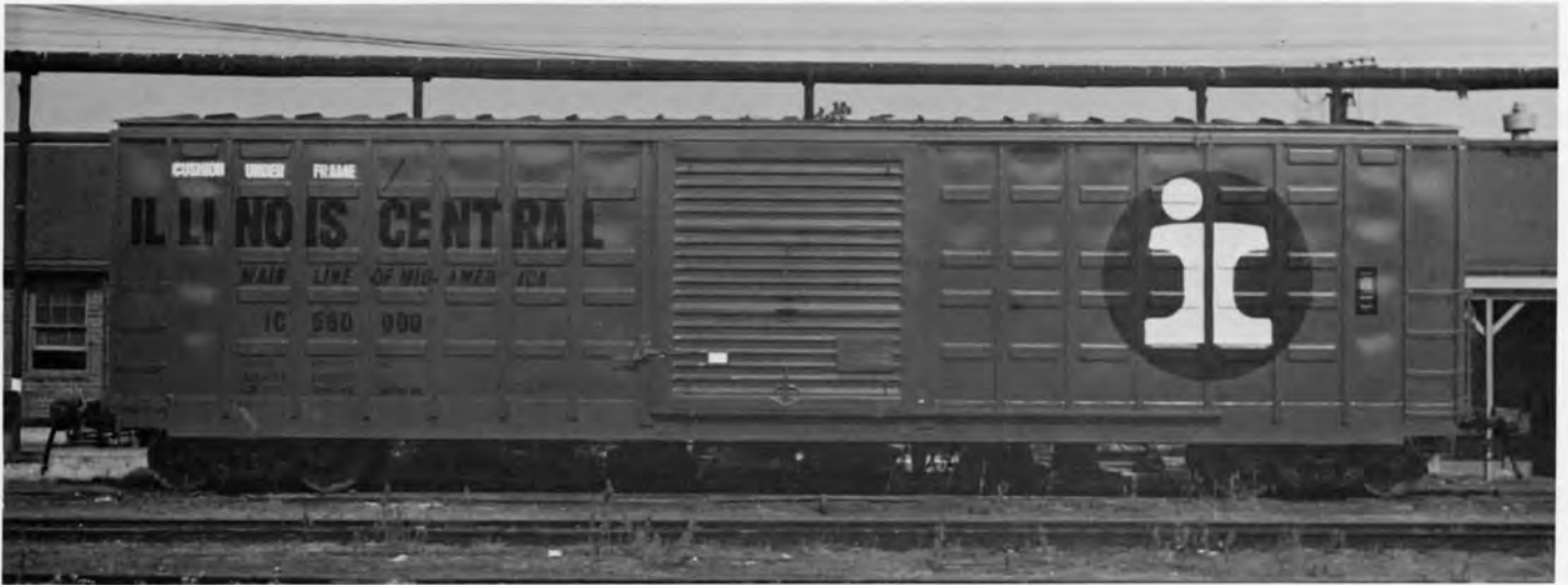
IC 580000 BOXCAR 50FT. PHOTO ICRR CENTRALIA SHOP EMPLOYEES - ICHS COLLECTION. 580000-580399 series cars built by the IC Centralia, IL car shop in 1970. Cars equipped with 4 belt DF-2 load devices and lading strap anchors. 70 ton capy car.
