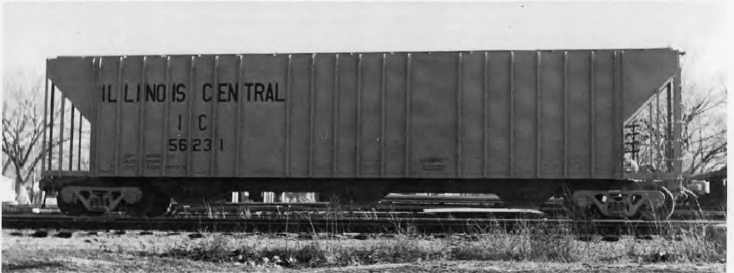
IC 56231 COVERED HOPPER PHOTO ICRR - ICHS COLLECTION. The 56000-56299 series cars were built by the IC Centralia, IL car shop in 1966.
