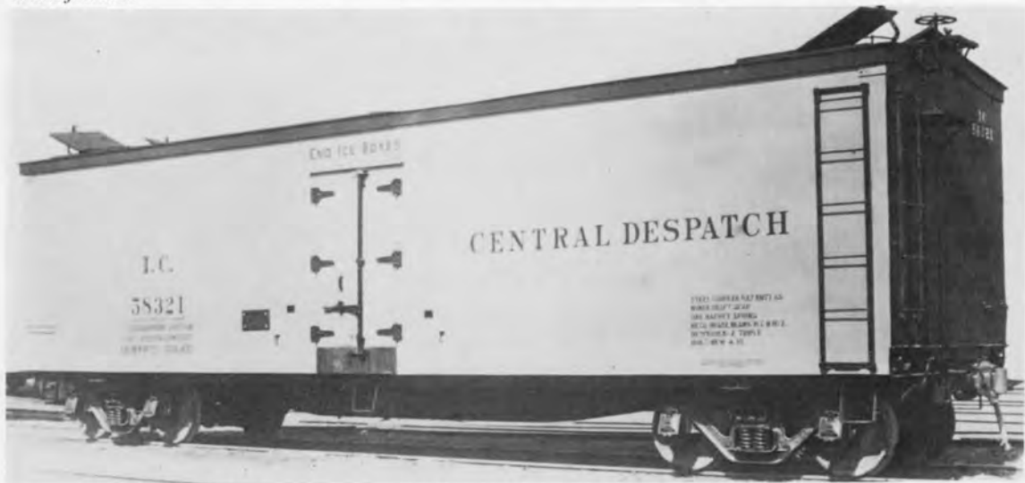
IC 58321 REEFER. PHOTO BY ACF - ICHS COLLECTION. The 58001-58900 series cars were built by ACF in 1915 at the Chicago, IL plant. The cars were 40 ton capy with fixed end ice boxes and steel underframes.
