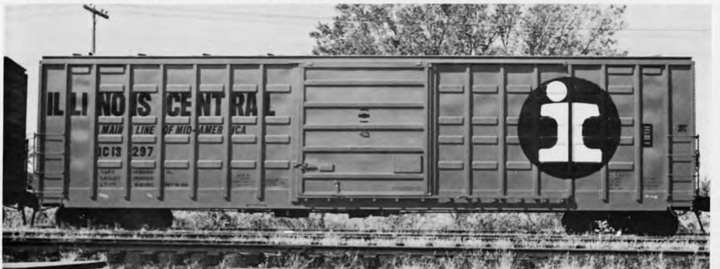
IC 13297 BOXCAR 50FT. PHOTO ICRR CENTRALIA SHOP EMPLOYEES - ICHS COLLECTION. The 13100-13399 series cars were built by the IC Centralia, IL car shop in 1969. Cars equipped with lading strap anchors and 4 belt DF-2 load devices.
