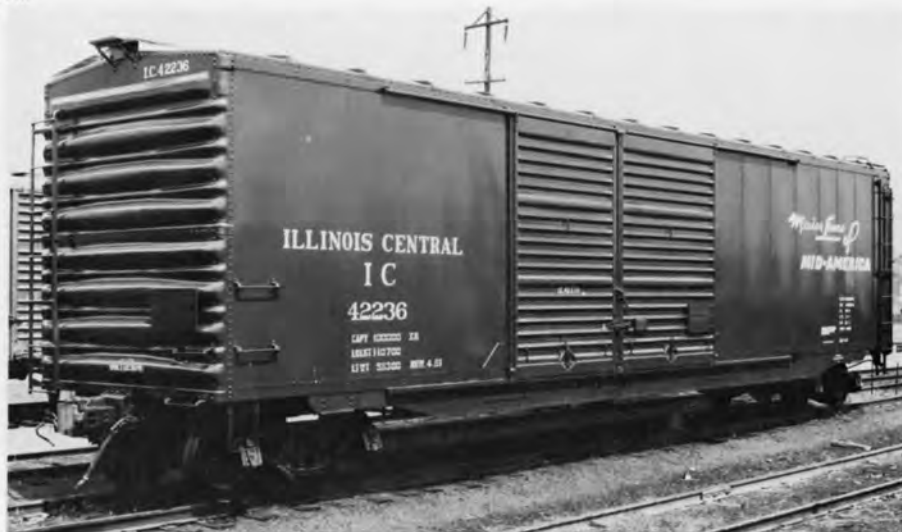
IC 42236 BOXCAR 50FT. PHOTO BY ICRR - ICHS COLLECTION. The 41800-42549 series cars were built by the IC Centralia, IL car shop in 1961. The cars were equipped with 2 \frac{1}{4} " wood flooring and assigned to auto parts service.
