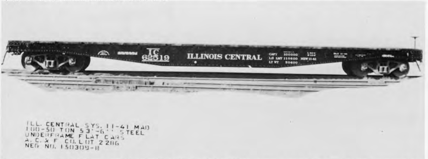
IC 62519 FLAT. PHOTO BY ACF - ICHS COLLECTION. The 62500-62599 series cars were built by ACF in 1941. The cars are 50 ton capy and 53 ft long. Assigned to general service.
