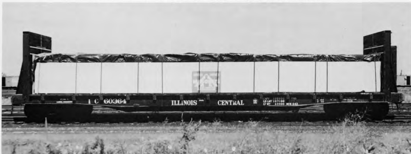
IC 60364 FLAT. PHOTO ICRR - ICHS COLLECTION. The 60300-60470 series cars were built by Bethlehem Steel Co. in 1963. The 50 ton capy bulkhead flats were assigned to wallboard loading.
