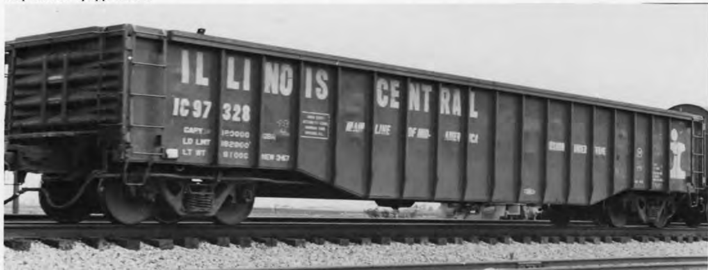
IC 97328 GONDOLA. PHOTO BY BRUCE MEYER - ICHS COLLECTION. The 97300-97349 series 100 ton, 52 ft covered gondolas were built by Greenville in 1967. The cars were equipped with three section removable roofs and assigned to steel service in the Chicago area for loading.
