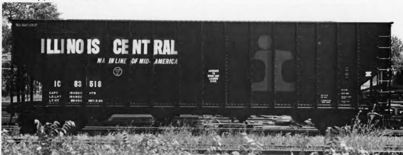
IC 83518 HOPPER. PHOTO BY ICRR - ICHS COLLECTION. The 83500-83599 series cars were built by the IC Centralia car shop in 1969. The 70 ton copy cars were assigned to wood chip loading only.
