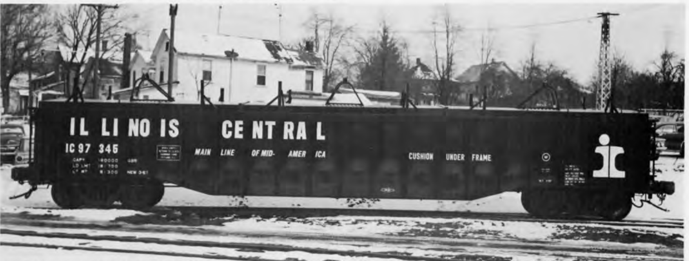
IC 97345 COVERED GONDOLA. PHOTO BY ICRR - ICHS COLLECTION. The 97300-97349 series covered gondolas were built by Greenville in 1967 for steel service in Chicago area. The cars are of 100 ton capy and are equipped with a three section removable roof.
