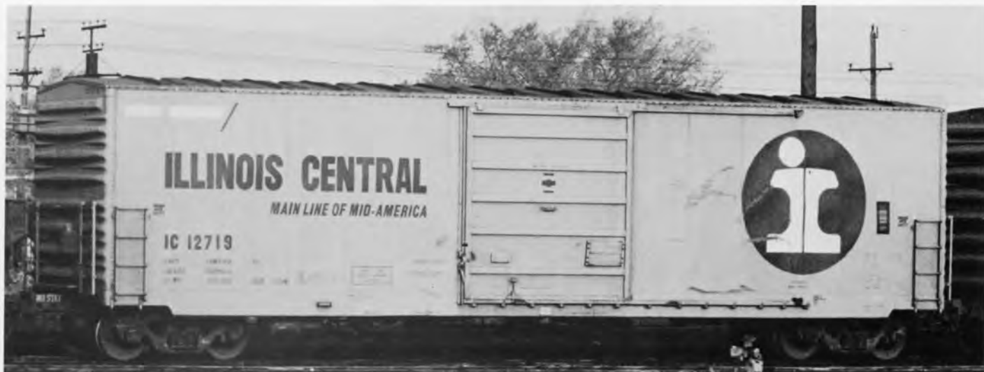
IC 12719 BOXCAR 50FT. PHOTO BY BRUCE MEYER. The 12700-12899 series cars built by G.A.T. Co. in 1968. Cars equipped with SL-2 load dividers and 2 3/8" nailable steel floors.
