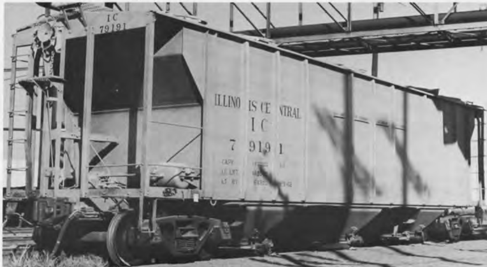
IC 79191 COVERED HOPPER PHOTO ALVINE DOYLE JR. ASSOCIATES, INC. - COLLECTION OF ELLIOT PARKMAN. The 79100-79199 series cars were 70 ton capy built by Pullman Standard in 1955 and were used for cement loading.
