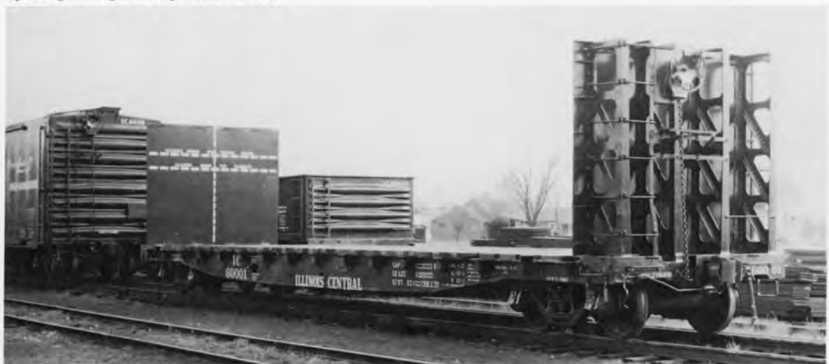
IC 60001 FLAT. PHOTO ICRR CENTRALIA CAR SHOP EMPLOYEES - DAVID DAISY COLLECTION. 21 cars at random from the 60000-60099 series of flat cars were equipped with 9 ft bulkheads for wallboard service. The other cars are 60018/60020/60022/24/26/29/42/51/54/56/61/65/66/81/86/87/88/91/92/93.
