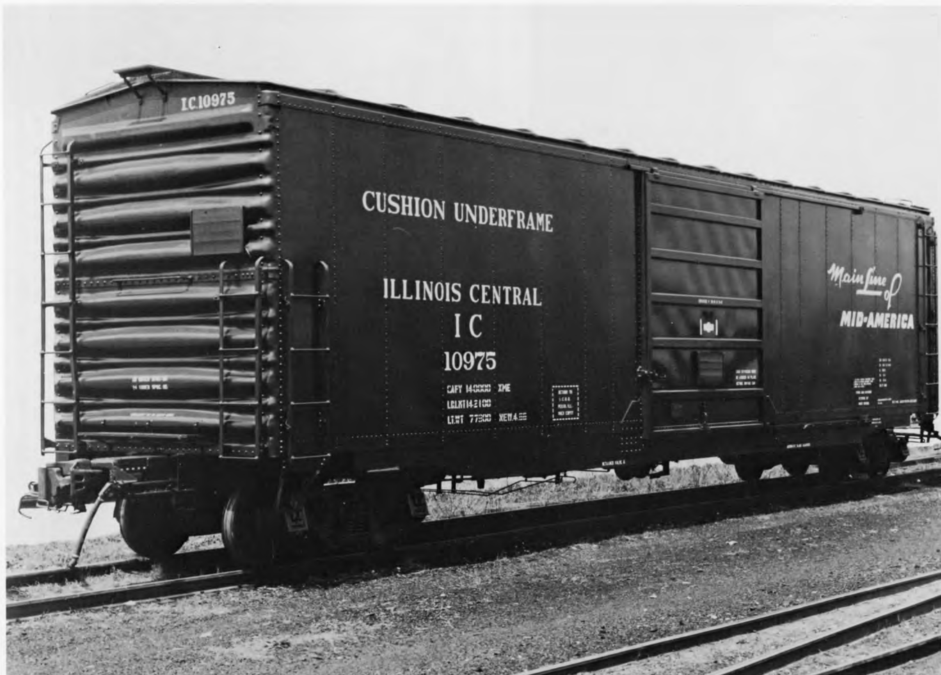
IC 10975 BOXCAR 50FT. PHOTO BY ICRR - ICHS COLLECTION. The 10975-10999 were built by the IC Centralia, IL car shop in 1966. The cars were equipped with 2 \frac{3}{8} " wood floor decking and Evans load dividers.
