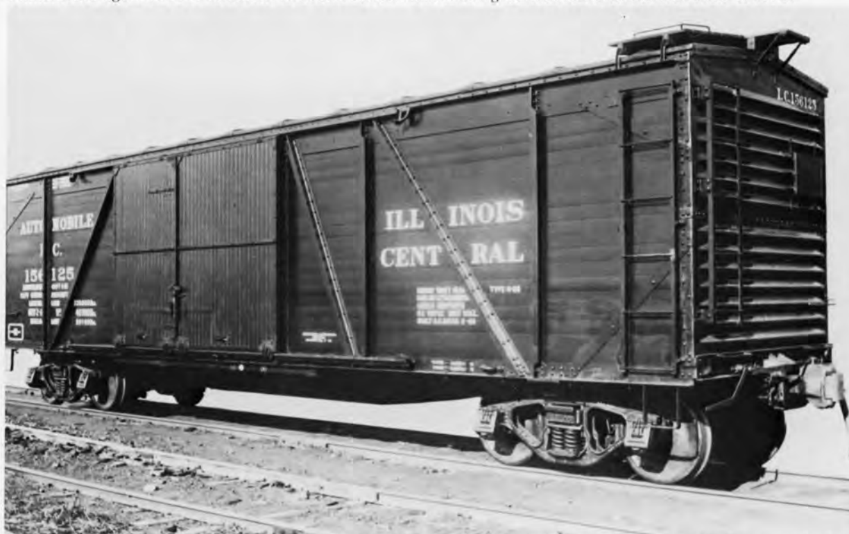
IC 156125 WOOD BOXCAR. PHOTO BY ACF - ICHS COLLECTION. The 156001-156500 series cars were built by ACF in 1925 at their Madison plant in Chicago area. Renumbered by the IC later to 11000 to 11974 series. Assigned to automobile service.
