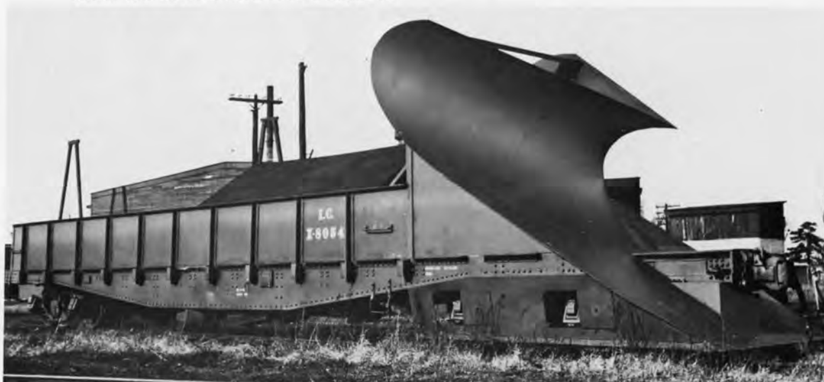
IC X8054 SNOW PLOW. PHOTO G.V. CARSON - ICHS COLLECTION. Part of a group of snow plows that the IC assigned to the northern half of Illinois and the Iowa Division. Converted by the IC from former flat cars, all were built to the same design. Most were equipped with headlights off retired steam engines.
