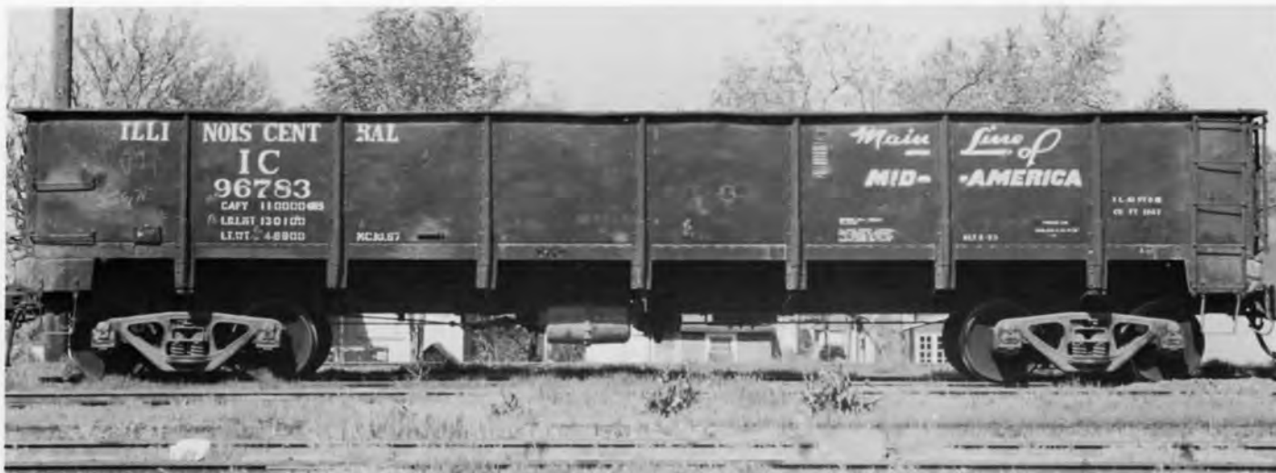
IC 96783 GONDOLA. PHOTO BY BRUCE MEYER - ICHS COLLECTION. The 96000-96929 series 41 ft, 50 ton solid bottom general service gondolas were rebuilt by the IC Centralia, IL and McComb, MS car shops in 1967 from the former 94000-95499 series drop bottom equipped cars.
