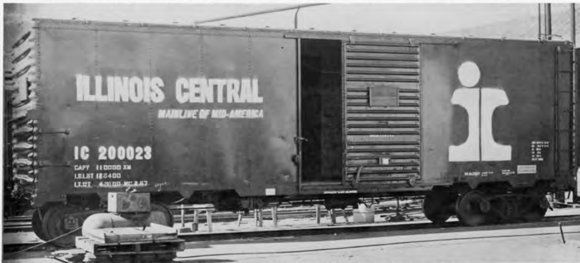
IC 200023 BOXCAR 40FT. PHOTO BY ICRR - ICHS COLLECTION. The 200000-200599 series cars were rebuilt by the IC McComb, MS car shop in 1967 from former 17000-20999 boxcars built between 1938 & 1940. General Service.
