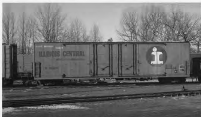
IC 150059. 50 FT. DD BOXCAR. 150025-150079. USRE 1972. 70 ton capacity.
