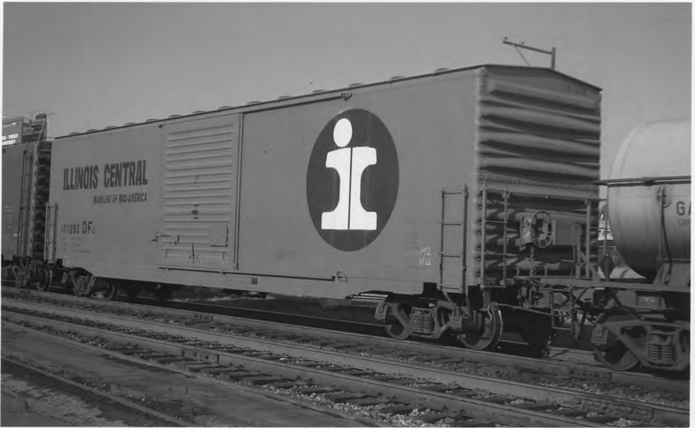
IC 11203. 50 FT BOXCAR. 11000-11299. ICRR 1967. 70 ton capacity.
