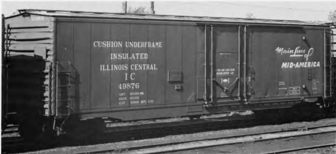
IC 49876 BOXCAR 50FT. PHOTO BY BRUCE MEYER. The 49770-49899 series cars were built by the IC Centralia, IL car shop in 1963. The cars were insulated, equipped with 2 \frac{3}{8} " Doweloc wood flooring and Evans load dividers.
