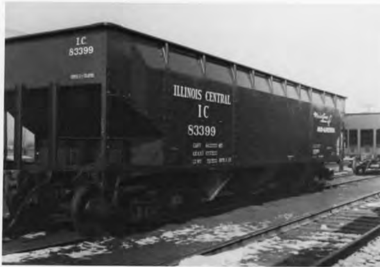
IC 83399 HOPPER. PHOTO ICRR - DAVID J. DAISY COLLECTION. The 82235-83499 series cars were built by the IC Centralia, IL car shop in 1960 & 1961. 70 ton capy.
