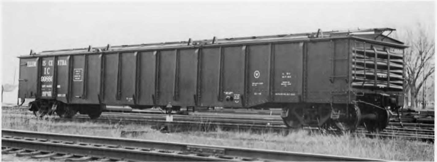
IC 99889 COVERED GONDOLA. PHOTO BY ICRR - ICHS COLLECTION. The 99800-99894 series cars were built by the IC Centralia, IL car shop in 1964 & 1965. The cars are 70 ton capy equipped with a three section diag. panel removable roof, four movable bulkheads and belt rails on the sides.
