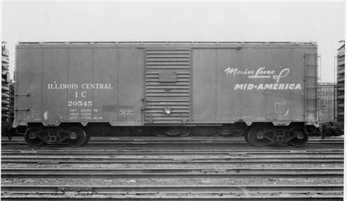
IC 20545 BOXCAR 40FT. PHOTO BY W.C. THURMAN - DAVID J. DAISY COLLECTION. The 20000-20999 series cars were built by Pullman Standard - Bessemer plant in 1940. Cars were upgraded by the IC McComb, MS car shop in 1966. This is one of 15 cars equipped with 5 belt DF loading devices for special loading.
