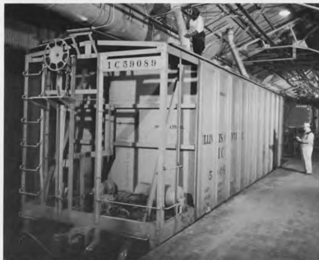
IC 59089 COVERED HOPPER PHOTO ICRR - HEDRICH-BLESSING - COLLECTION OF ICHS. The 59085-59096 series of cars were built in 1960 by G.A.T.X. and were part of the 59010-59196 single bay airslide covered hoppers owned by the IC. Cars were assigned to flour, sugar and dry chemical service.
