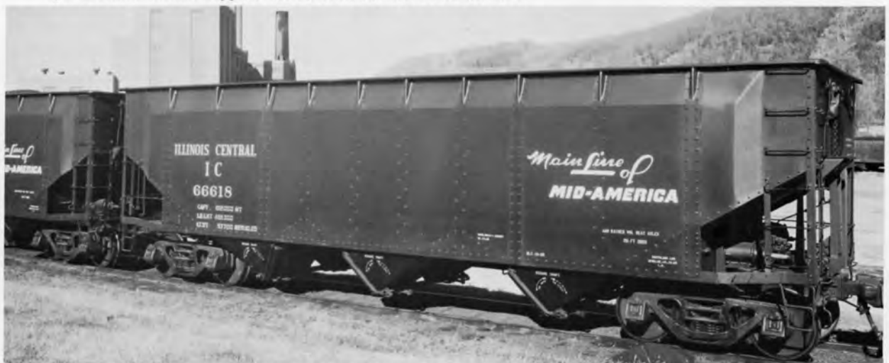
IC 66618 HOPPER. PHOTO HEDRICH-BLESSING (ICRR) - ICHS COLLECTION. The 65300-66699 series cars were built by the IC Centralia, IL car shop. The 70 ton hoppers were the second of three orders for hoppers in the 65000-67999 series.
