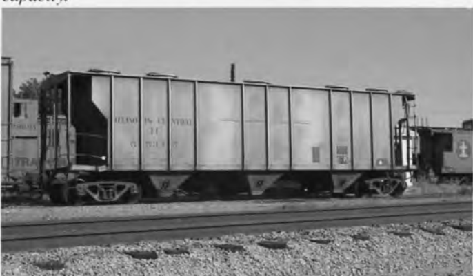
IC 55345. COVERED HOPPER. 55300-55499. Pullman Standard 1965. 70 ton capacity.
