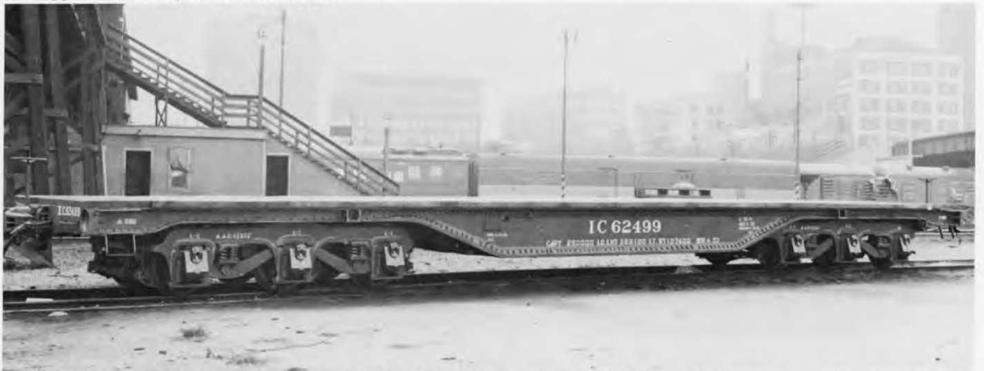
IC 62499 FLAT. PHOTO BY ICRR - ICHS COLLECTION. #62499 was built by the IC Centralia, IL car shop in 1953. The 125 ton, 53 ft flat car is equipped with a cast underframe and 3" oak wood deck. The underframe was cast by General Steel.
