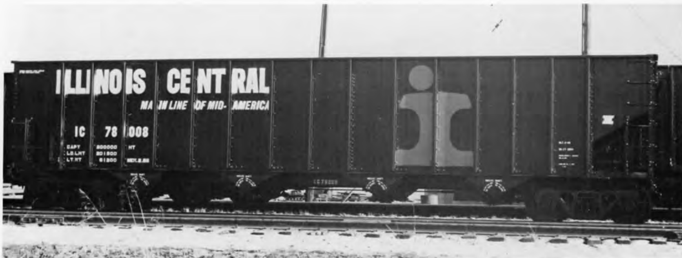
IC 78008 HOPPER. PHOTO ICRR - ICHS COLLECTION. The 78000-78999 series cars were built by the IC Centralia car shop in 1968. They were the first 100 ton copy hoppers owned by the IC.
