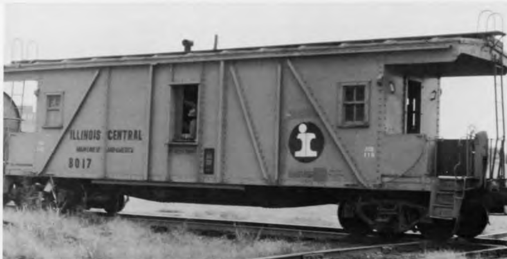
IC 8017 TRANSFER CABOOSE. PHOTO BY DENNIS CONNIFF - DAVID J. DAISY COLLECTION. The 8000-8020 cabooses were rebuilt by the IC in 1948 from former 10000-13958 wood side boxcars. The wood sides on the cabooses were replaced by steel sides starting in the 1960s.
