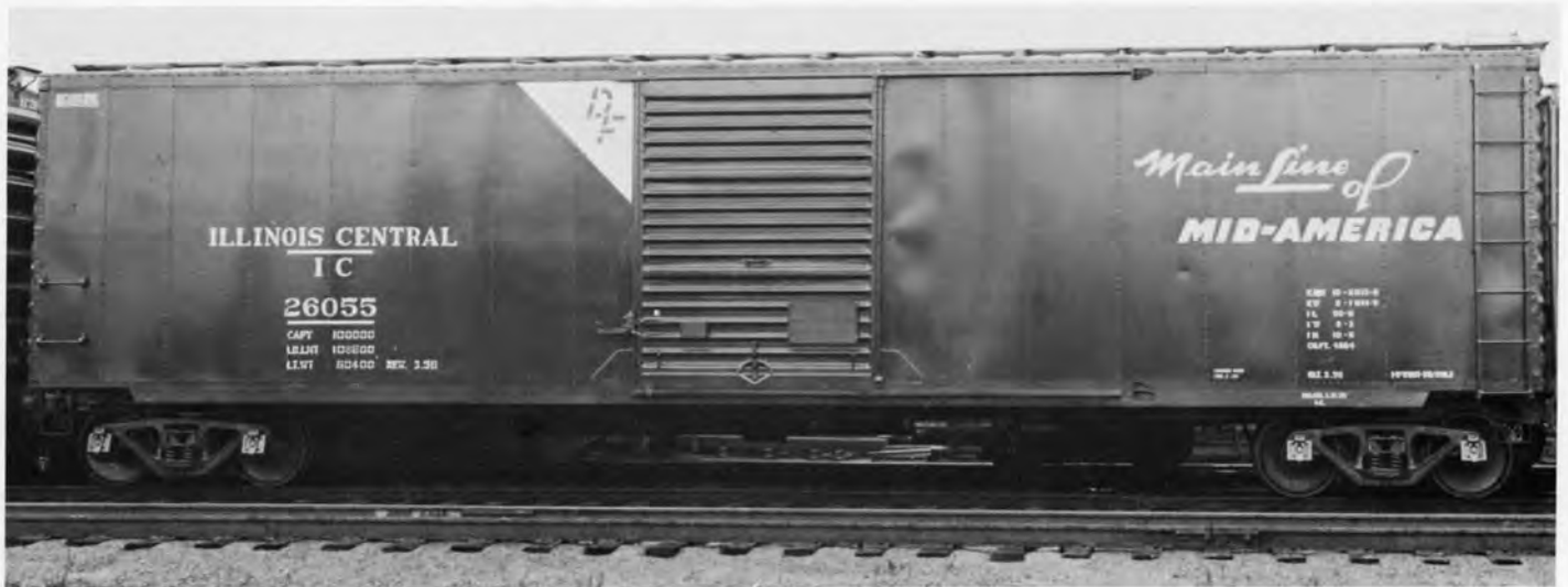
IC 26055 BOXCAR 50FT. PHOTO BY ICRR - ICHS COLLECTION. The 26000 - 26099 series cars were built by the IC Centralia, IL car shop in 1956. The cars were equipped with 9 belt DF loading devices and 1/4" wood floor decking.
