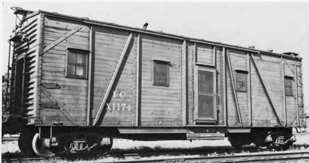
IC X1174 BUNK CAR. PHOTO G.V. CARSON - ICHS COLLECTION. Former wood side boxcar that the IC converted to a bunk car.
