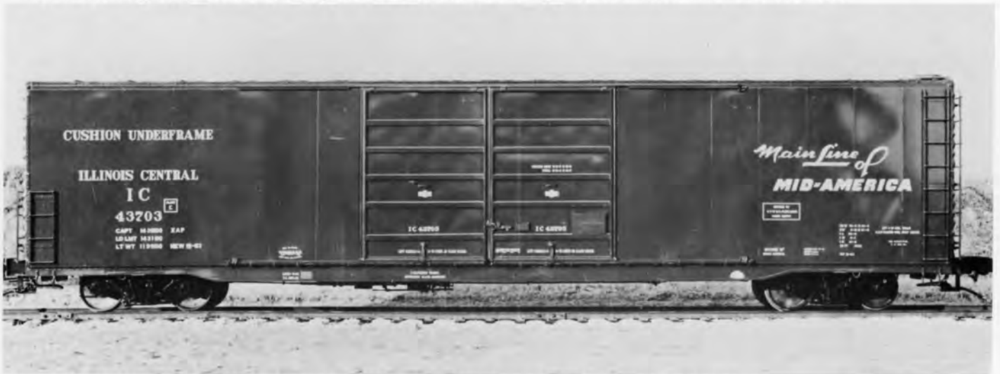
IC 43703 BOXCAR 60FT. PHOTO BY ICRR - DAVID DAISY COLLECTION. The 43700-43749 series cars were built by Thrall in 1963. Cars are equipped with 1/4" nailable steel flooring. Assigned to GTW RR for loading auto axles at Pontiac's Flint, Michigan auto plant.
