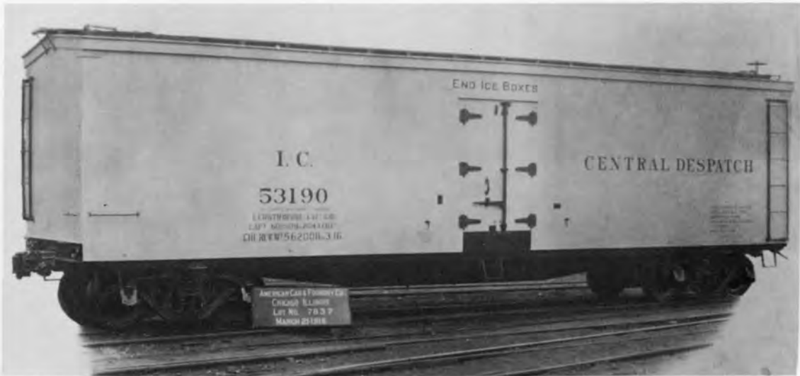
IC 53190 REEFER. PHOTO BY ACF - ICHS COLLECTION. The 53001-54000 series cars were built by ACF in 1916 at the Chicago, IL plant. The cars were 40 ton capy with fixed end ice boxes and steel underframes.
