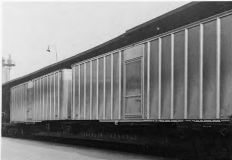
IC 900 FLAT CAR. PHOTO ICRR - ICHS COLLECTION. IC Flex-van flat cars were used for carrying U.S. Mail vans. The flats were equipped with steam & signal lines for use in passenger service or freight service.
