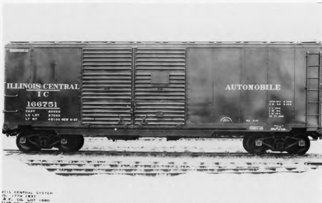
IC 166751 BOXCAR 40FT DD. PHOTO BY ACF - ICHS COLLECTION. The 166500 - 166999 series cars built by ACF Chicago in 1937. Renumbered to 35500-35999 in 1938. Cars equipped with auto loading devices. Cars renumbered again in 1941 to 36500 to 36999 series. Auto loading devices removed between 1950 & 1952.
