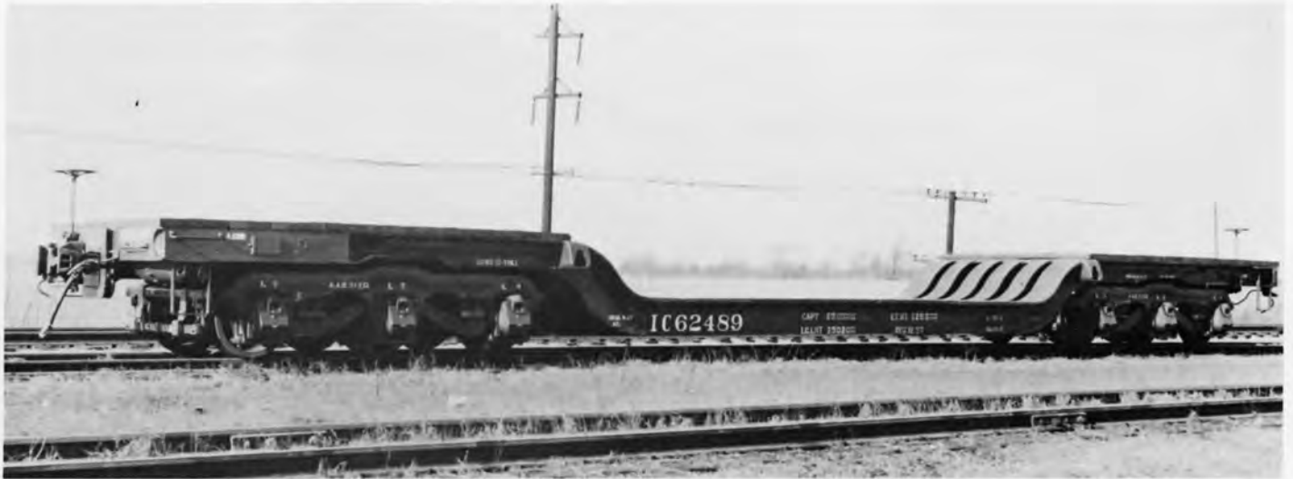
IC 62489 FLAT. PHOTO BY ICRR - ICHS COLLECTION. #62489 was built by the IC Centralia, IL car shop in 1957, 125 ton capy, 57 ft depressed center flat car. The cast underframe was built by General Steel Casting in East St. Louis, IL. Car equipped with cast steel loading floor and end of car cushion devices.
