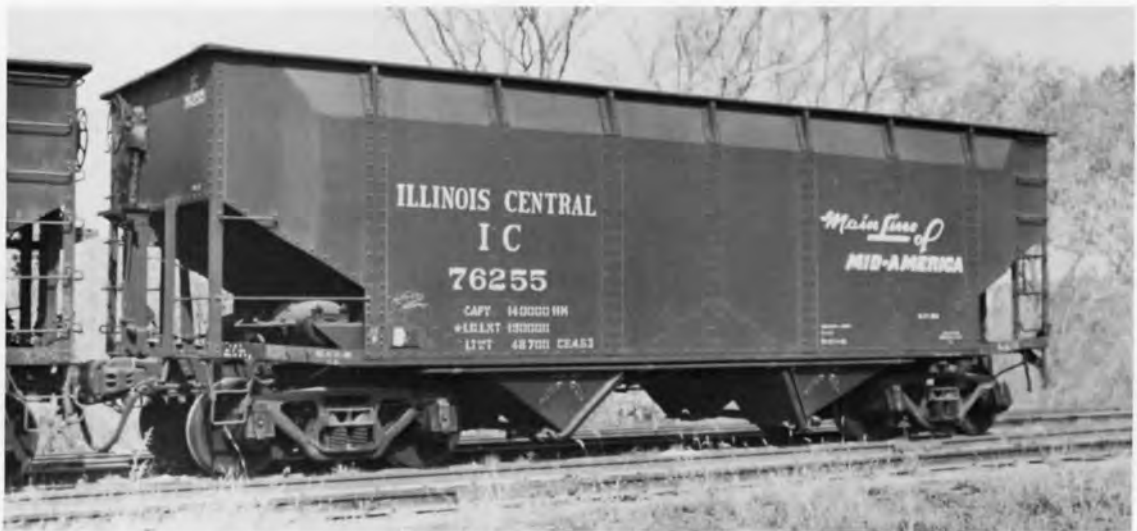
IC 76255 HOPPER. PHOTO JAY WILLIAMS - ICHS COLLECTION. The 76000-76999 series 70 ton cars were built by the IC Centralia, IL car shop in 1963. These hoppers were the second of three orders built of the 75000-77999 hoppers the IC built between 1962 & 1964.
