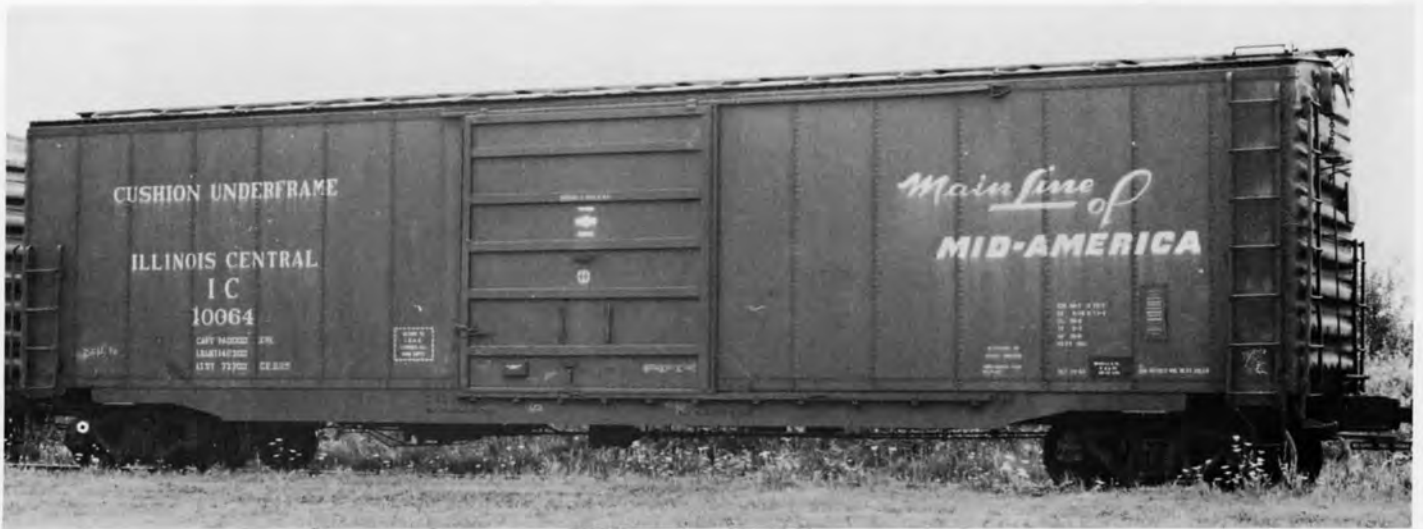
IC 10064 BOXCAR 50FT. PHOTO BY BRUCE MEYER. The 10000-10199 series cars were built by the IC Centralia, IL car shop in 1964. The cars are 70 ton capy equipped with nailable steel floors and 3 DF-2 partial belts load devices.
