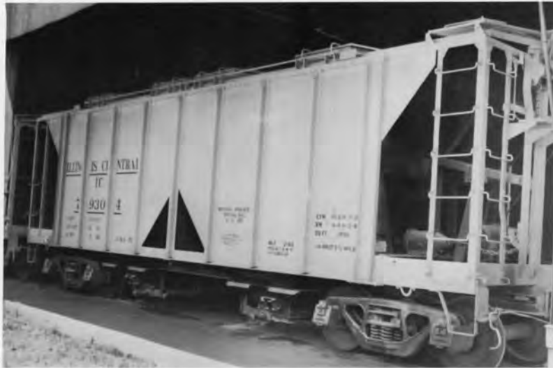
IC 79304 COVERED HOPPER PHOTO BY ICRR - ICHS COLLECTION. The 79300-79311 series cars were built by Pullman Standard in 1953 with 70 ton capy.
