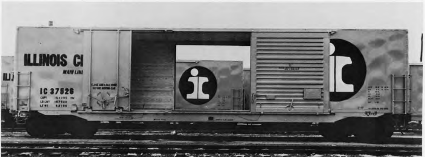
IC 37526 BOXCAR 50FT. PHOTO ICRR - ICHS COLLECTION. This car is part of the 37500-37699 series built by Pullman Standard in 1967 and equipped with combination doors and 2 3 / 8 " Durawood floor decking.
