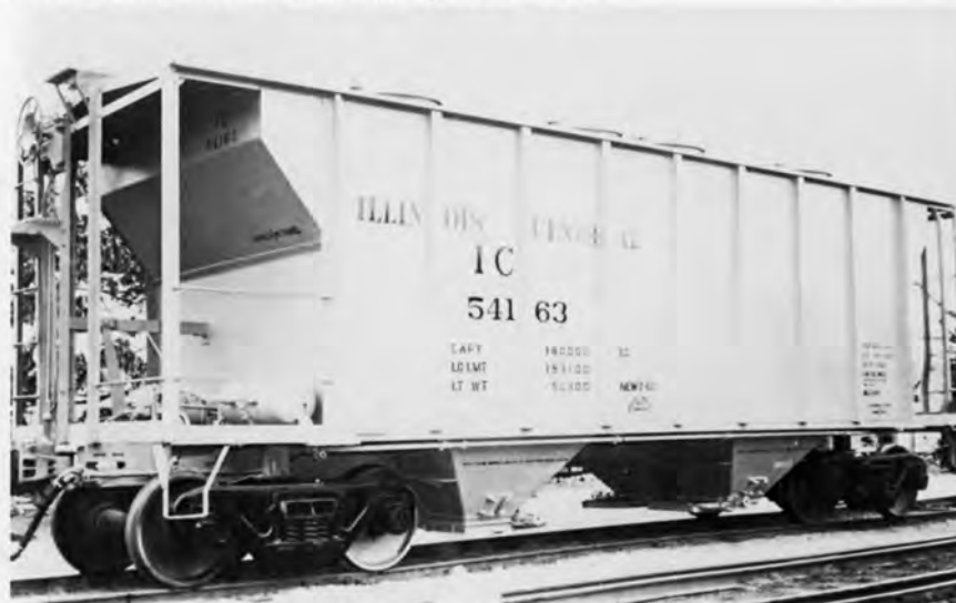
IC 54163 COVERED HOPPER PHOTO BY ACF - ICHS COLLECTION. The 54150-54249 series cars were built by ACF in 1960 with 70 ton capy, most were assigned to cement service.
